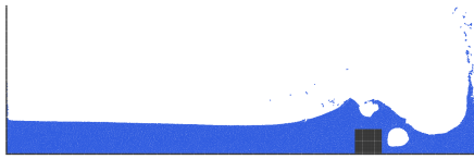
Figure 15: 2D dam breaking simulation with SPH
